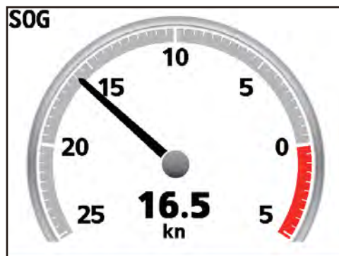
Symbol Location: Right (The pointer rotates counterclockwise as ship's speed increases.)
