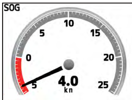
Astern SPD Scale: 5 kn Ahead SPD Scale: 25 kn Symbol Location*: Left (The pointer rotates clockwise as ship's speed increases.)
