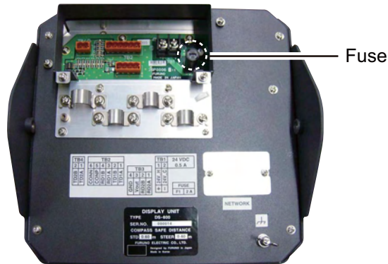
Fuse location (Rear panel: cable cover removed)
