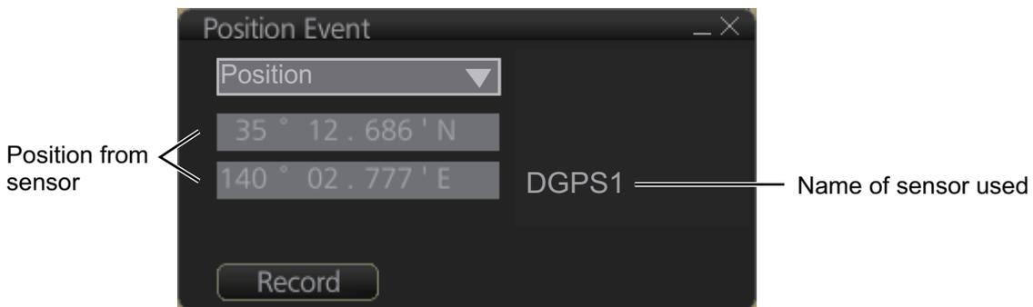
The [Position Event] window shows the position at the moment the [Record] button is clicked. The position is recorded to the [Voyage] log.
