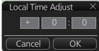
2. Enter the time difference between the local time and the UTC time, in hours and minutes. Use the button on the left to select the time offset direction. Select "+" if the local time is ahead of the UTC time, or "-" if it is behind the UTC time.
