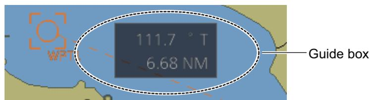
**Note 2:** The bearing and range of the waypoint can be adjusted as shown below.
