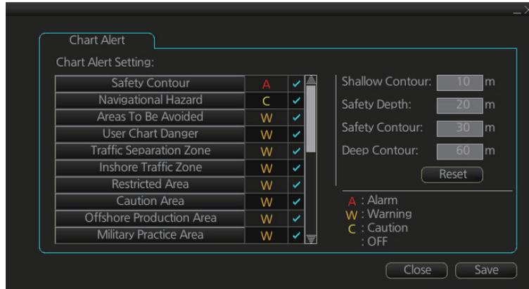
2. Click a letter indication to select the type of alert, warning or caution, to receive for the given chart object. [Safety Contours] is fixed to "A" (Alarm).
