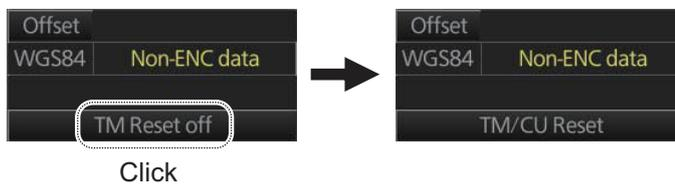
When the TM reset is disabled, change the chart scale with the scrollwheel and scroll the chart by drag and drop. The own ship information box shows the indication "TM Reset off". To restart true motion, click the indication. When own ship moves off the screen the box shows the indication "Ship off screen". To restart true motion, click the indication.
