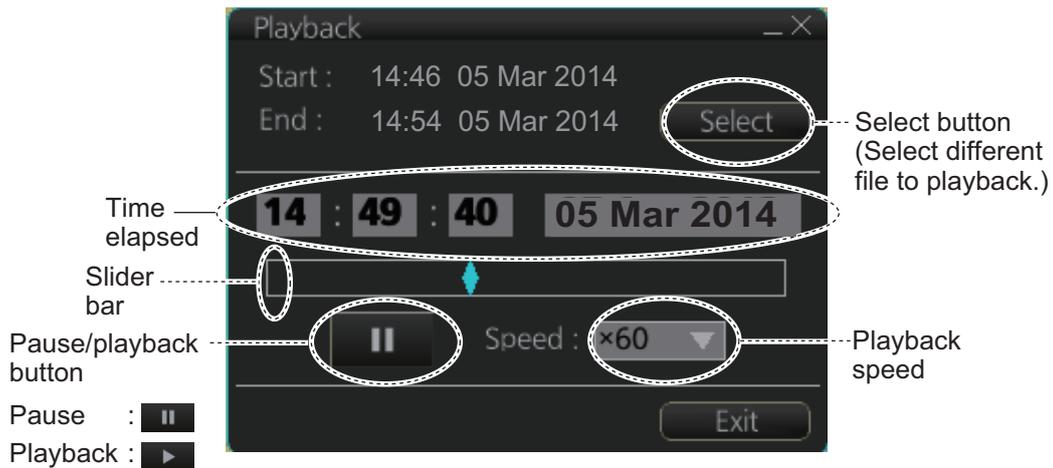
All your ship's movements and chart-related operations during the time period selected are plotted on the screen and the screen shows the message "PLAYBACK". To stop playback and return to the normal display, click the [Exit] button. The message "Please Restart ECDIS for using other functions without playback." appears. Click the [Restart] button to restart ECDIS.
