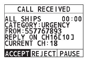
ACCEPT: Select the soft key to continue with the call and switch to the requested channel.
