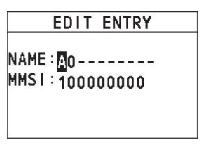
Step 6 After you finish entering the information, press the **Menu/DSC** control to save the setting and return to the previous screen.
