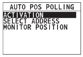
Step 3 Select "ACTIVATION". The "ACTIVATION" page appears on the screen. The screen shows two soft keys: "START" and "STOP".
