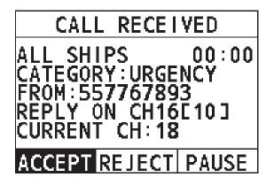
• ACCEPT: Select the soft key to continue with the call and switch to the requested channel.
