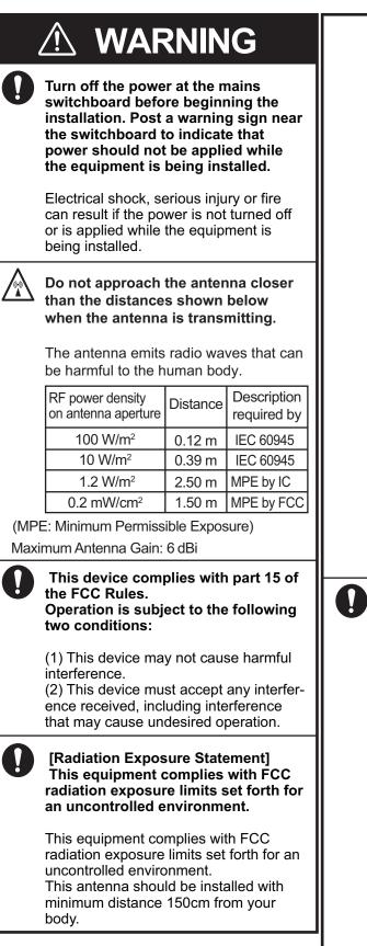
This transmitter must not be co-located or operating in conjunction with any other antenna or transmitter.
