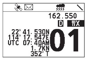
In weather mode, you can rotate the Menu/DSC to select a NOAA channel to monitor. What you selected would be mark as last used weather channel.
