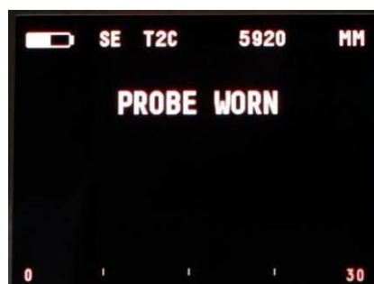
Probe Worn Message on Measurement Screen.
