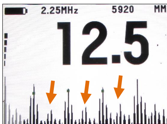
Flat, new steel 12.5mm thick with blind hole.
