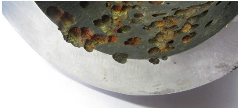
Large Corrosion Pits.
