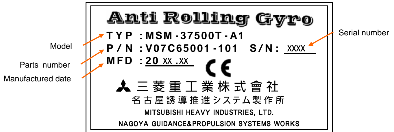
Figure 2-6 Nameplate for the ARG unit
