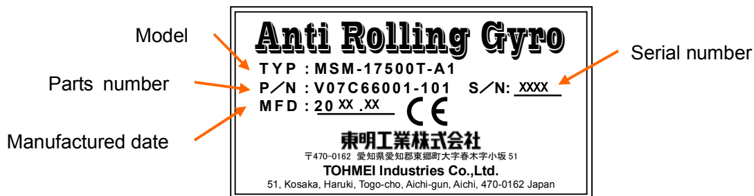
Figure 2-6 Nameplate for the ARG unit
