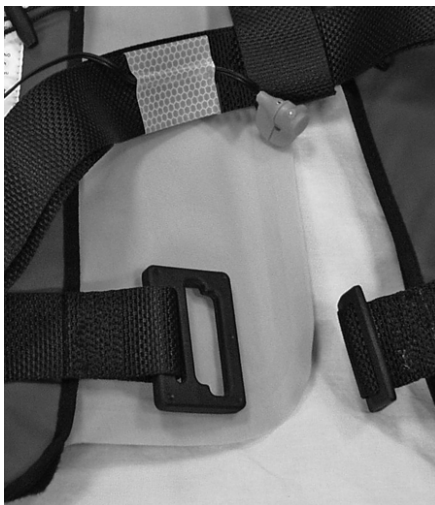
Example of sensor taped to back strap of lifejacket to ensure immersion
