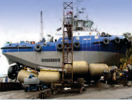
Draft reduction for newly constructed tugboat launching using Salvage Pontoons 40,000 lbs. and Salvage Pontoons 70,000 lbs.
