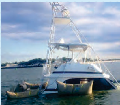
60 ft Yacht salvage using EFB-4000's and EFB-6000's. Photo Credit: Sea Tow Ocean City - Maryland , USA
