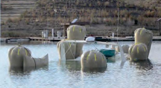
Raising Wayne Newton's yacht with Professional Lift Bags 12,000 lbs. and Enclosed Flotation Bags 6,000 lbs. Metropolitan Marine Solutions, Arizona, USA.
