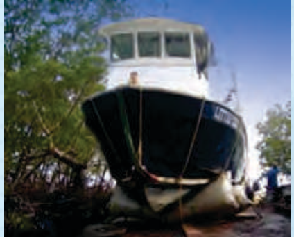
Enclosed Flotation Bags 6,000 lbs. used as pneumatic jacks/skids to remove and re-launch a grounded crewboat.
