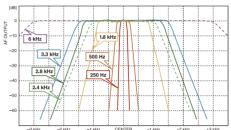
\* 6 kHz: Wide standard filter 2.4 kHz: Normal (Narrow for AM) standard filter
