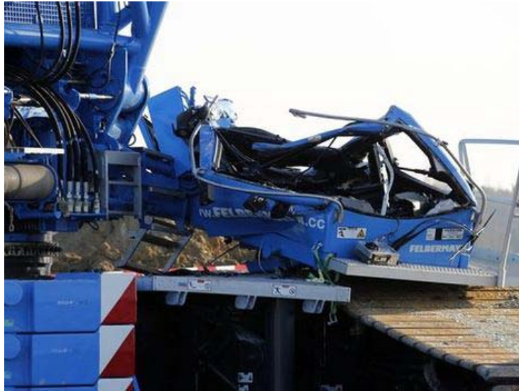
Crane cab destroyed by turbine blade landing on top of it
