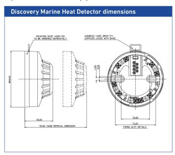
${\it Note:}$  Should be used with Deckhead Mounting Box - Part No. 45681-217 if ingress protection is required.
