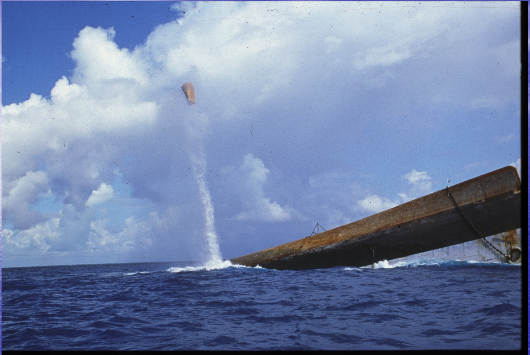
Professional 50,000 lb lift bag rocketing 150 ft. into the air after rigging failure on (Speigel Grove).
